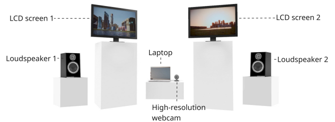
Figure 3: Technical setup of the installation with LCD displays, loudspeakers, computer, and camera.
