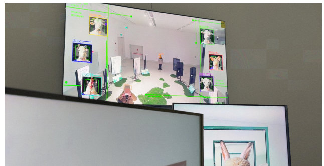
Figure 2: On-site Diagram of Camera and AI Recognition Technology Capturing Viewer Positions and Facial Features
